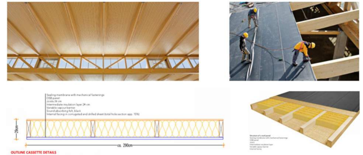
Figure 8.1: Timber Cassette System – Typical Details
