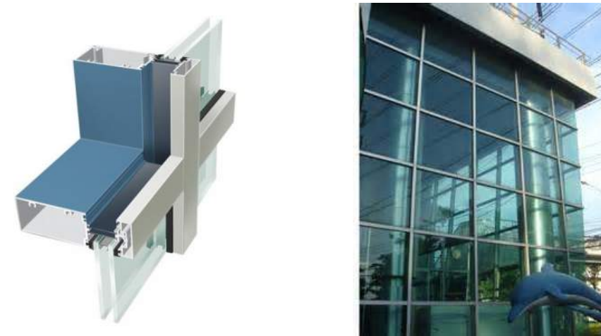
Figure 8.4: Typical Façade System for Glazing
