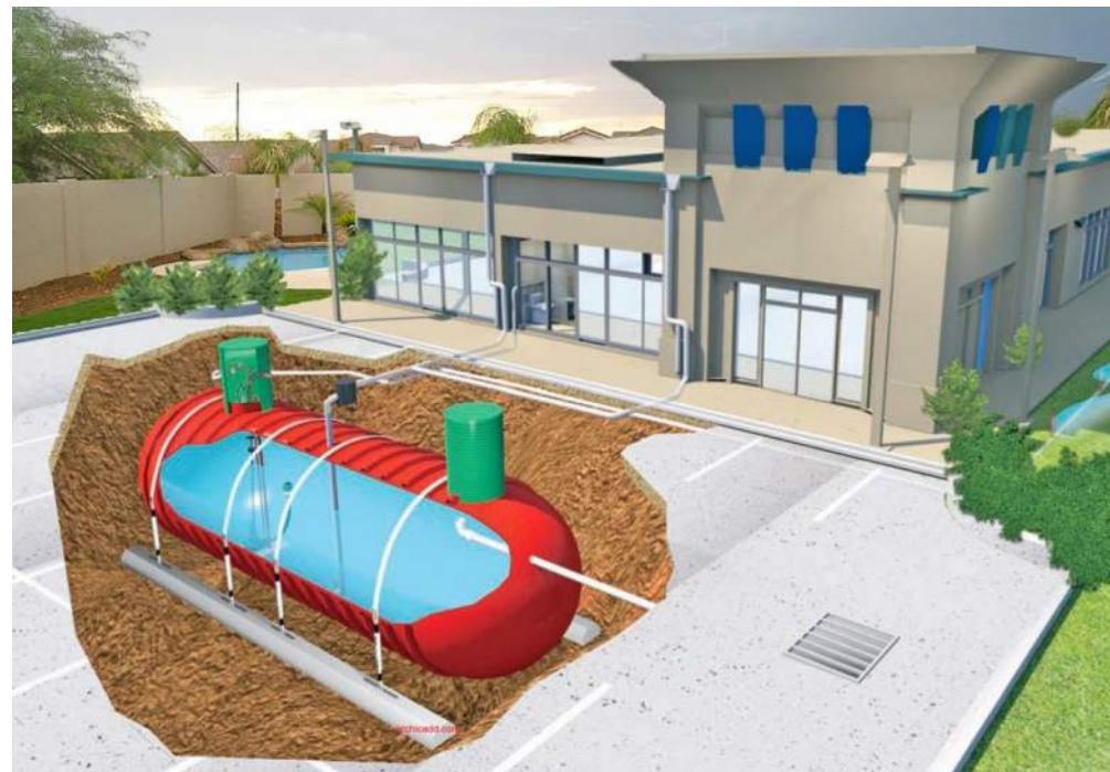
Figure 9.5 – Indicative Rainwater Harvesting Layout
